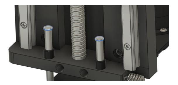
Fit the hose to the X hose support and lower hose support sliding it securely over each hose support.
