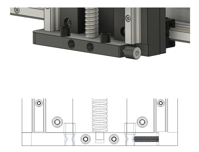
Insert the dust boot supports into the slider support from above (ensure the Z is in home position). Insert the dust boot height adjuster screw.
