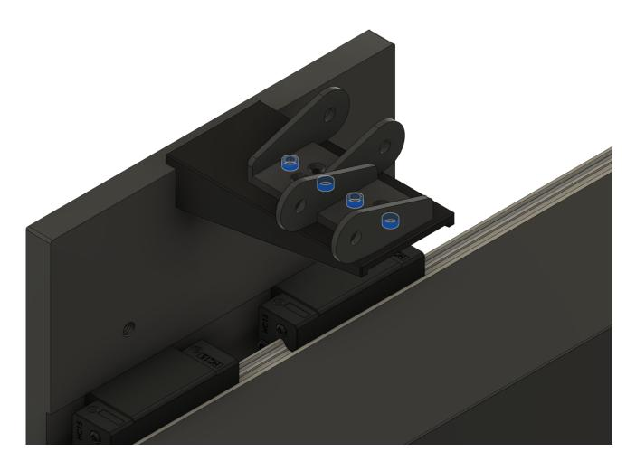
Remove the 2 rear drag chain support screws
