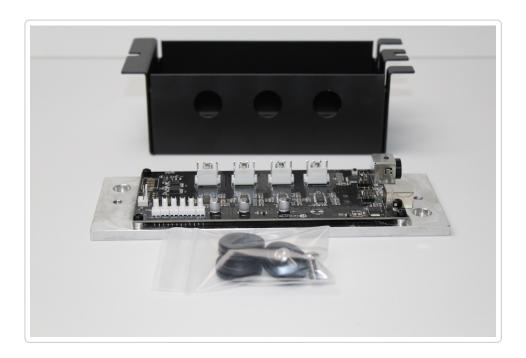
Install the controller on the back of the X-rail. The controller is connected with two M6x12mm screws (button head).
