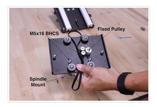
Tighten these screws down at this point in the assembly. Using some thread locker will help keep them secure and reduce the chance of vibration causing the screws to become loose.
