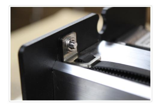
Working your way towards the other end of the Y-Axis Rail, run the belt between the rail and the flanged idlers. Pushing from both sides of the idler, force the belt up and towards the idler. You can also use the 1.5mm hex key to lift the belt between the idlers. Once the belt is accessible, wrap around idler.
