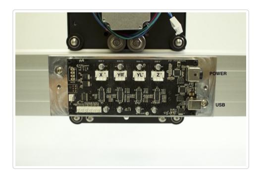
When installing the controller, ensure the orientation matches what is shown in the picture. The USB and Power ports should be facing to the right (as viewed from the same direction as the picture)
