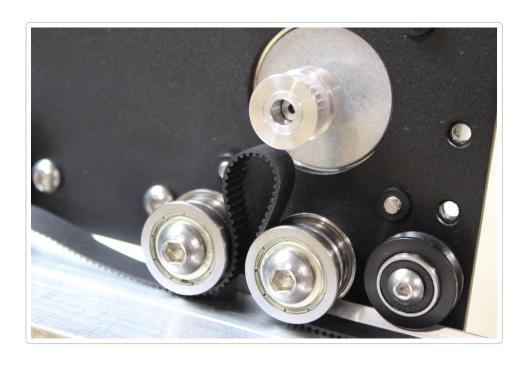
Using another M5x10mm screw, tension the belt clip against the front of the machine.
