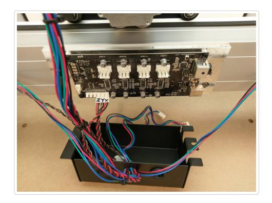
If you are installing homing switches at this time, route those through the port opening and to their connection points. Notice the orientation of the cables and the order (X/Y/Z from right to left).
