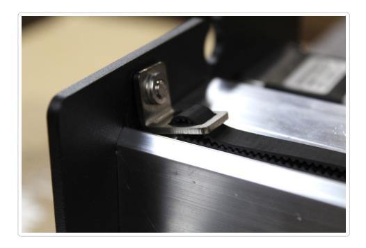
After the belt has been run through the clip, ensure the teeth have interlocked with each other and there is roughly 2 inches (50mm) of underlapping belting.
