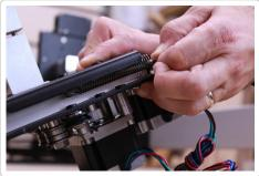
Turn the X/Z Carriage on its other side and attach second spring in identical manner as shown in the image below.
