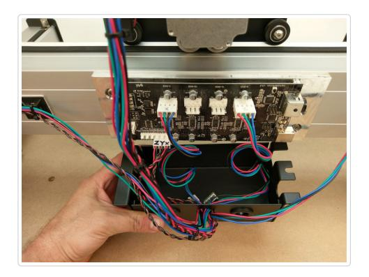
Attach the X and Z axis stepper motors to their respective ports (labeled on the silkscreen as well).
