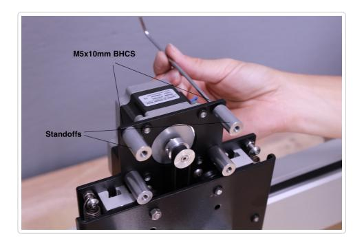
**PROTIP:** It will be easier to install the plate if you do not tighten the standoffs at this time.
