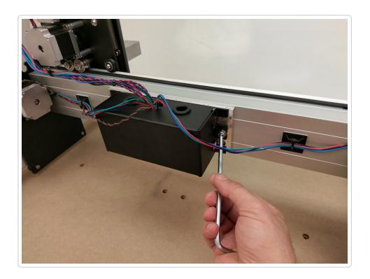
After your wires have been connected to the correct ports, install the enclosure cover using the included M6 x 8mm Socket Head Cap Screws (one on each side).
