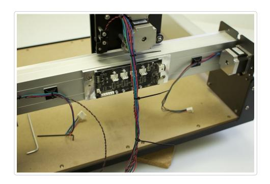
The X/Z Assembly works best by using 4 of the zip-ties to create a wire bundle, with a zip tie placed ever 4–6 inches down the bundle.
