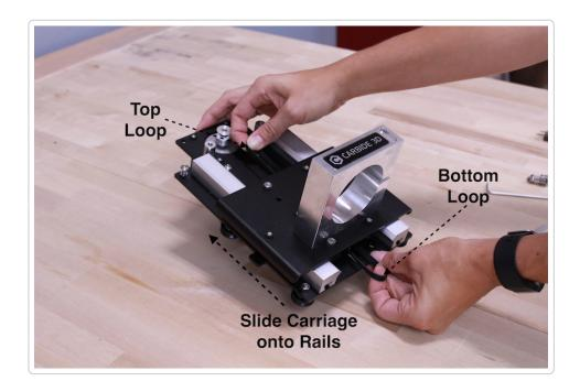
Slowly pull the bottom portion of the belt and loop it over the Idler as shown.
