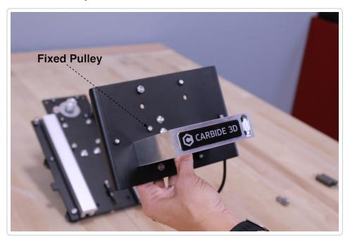
Align the spindle mount with the bottom set of through holes on the z-carriage. The Carbide 3D logo should go right side up, but the position of the pocketed hole on the spindle mount does not matter (left or right is fine).
