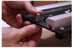
Carefully remove the nut while ensuring the remaining components stay on the bolt. Insert the bolt through the slot located at the bottom of the plate - shown in the image below. Secure in place by finger-tightening the nut on the opposite side of the X Carriage.
