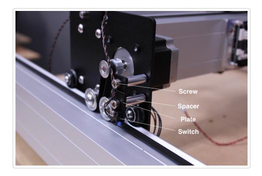
**PROTIP:** Before you can use the homing feature, homing will need to be enabled in the software configuration.
