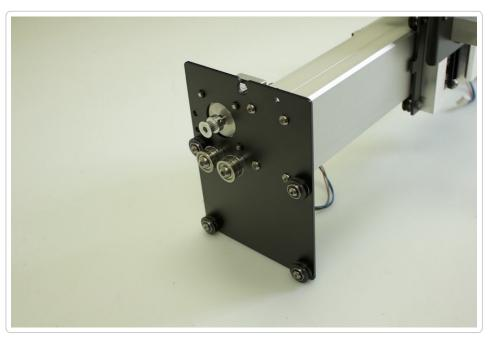
In this step, you will be installing the extrusion with the threaded mounting holes on the back side!
