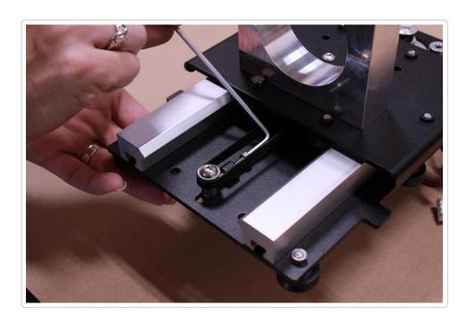
Use the hex wrench to tighten the Tensioning Screw as shown in the image below. As the Tensioning Screw is tightened, it will push on the Idler Assembly.
