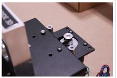
Ensure that you have only finger-tightened the Idler Assembly before tightening the Tensioning Screw.
