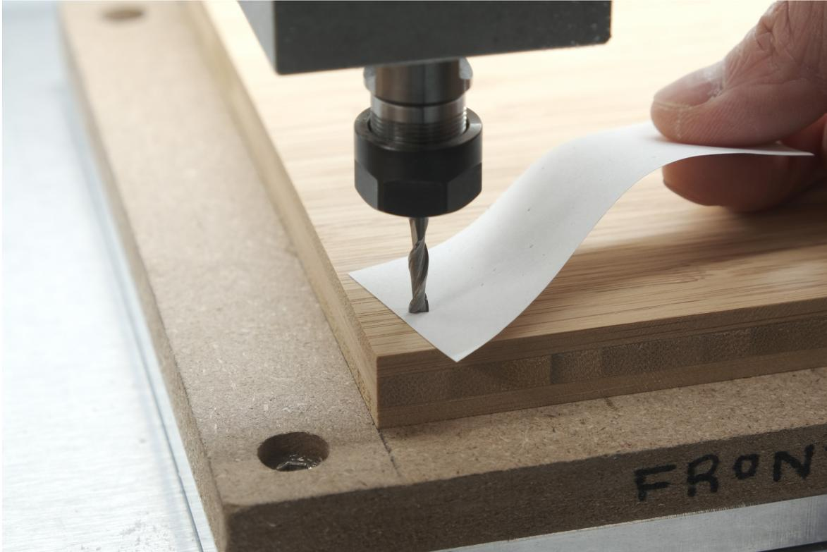
6. Very slowly, and with a very small increment, resume lowering the cutter towards the material. Simultaneously, begin moving the paper back and forth across the top of the material.
