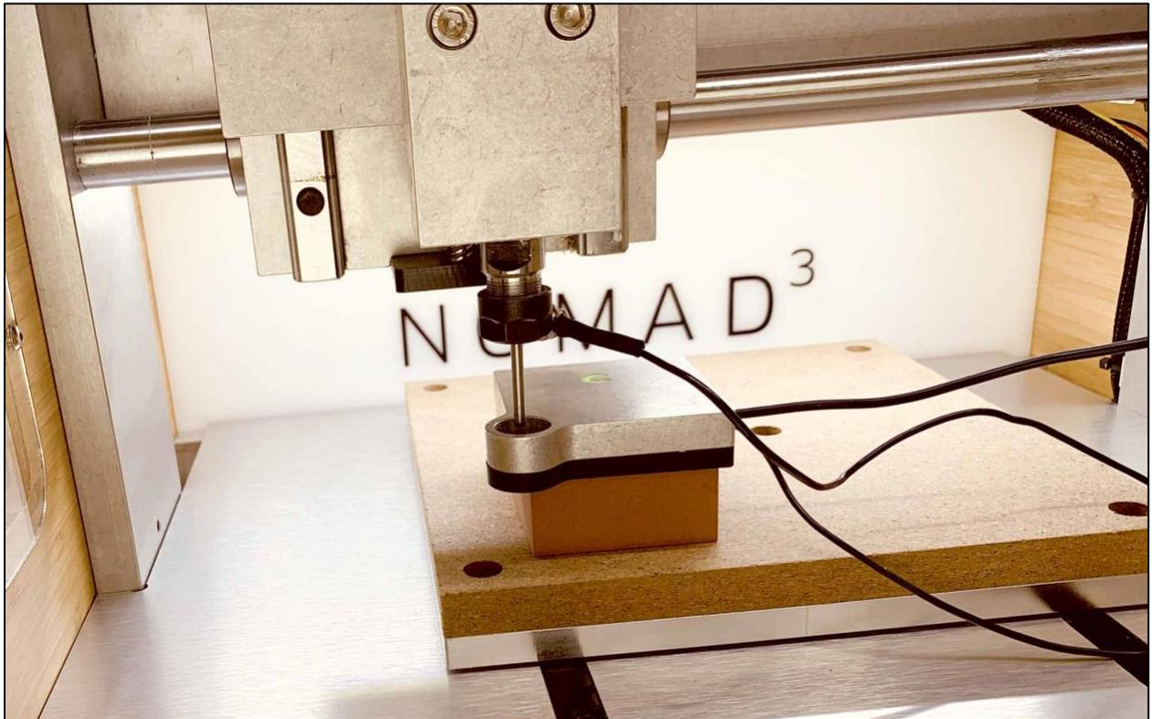
5. Attach the BitZero V2's magnetic grounding clip to either the collet nut or the probing pin in the spindle.
